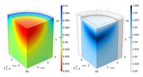
**Figure 1:** Simulation results from a simulation of a stack of 450 dielectric elastomers. The electrodes are applied in the middle of the stack covering 64% of the total area. The picture to the left displays the stretch ratio in the z-direction, and the ratio of the normalized electric field to the initial electric field is displayed on the picture to the right.
