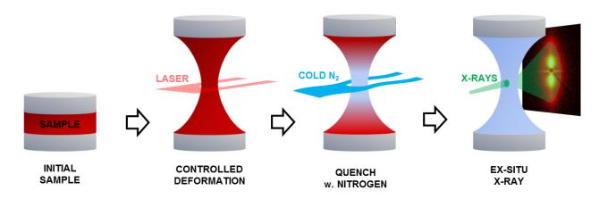
Figure 1: Experimental protocol for studying the correlation between extensional rheology and final morphology of polymeric fibers.
