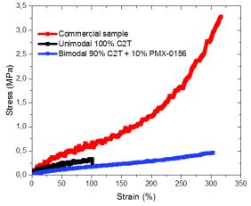
Figure 1: Stress-strain curves at room temperature and at strain rate of  $0.01 \text{ s}^{-1}$
