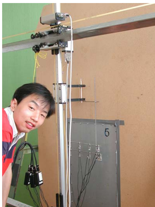
Yang Liu and his experimental setup with a robot borrowed from Brüel & Kjær and an array of p - u sound intensity probes borrowed from Microflown.
