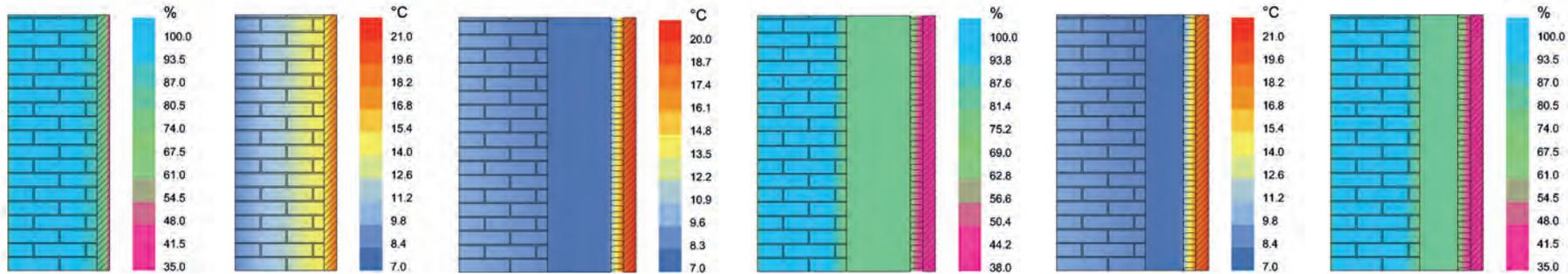
Results from Delphin analysis: scenario: Original wall and wood plate. Left: moisture build up. Right: temperature/heat loss (average over 5 years).
