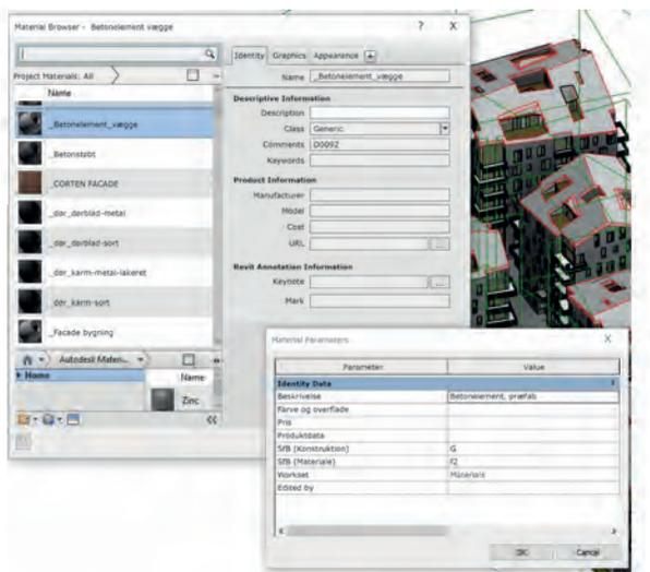
Screenshot from Revit, error checking of the model prior to the LCA calculation process
