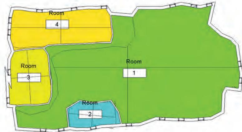
A hand sketch (left) and a fully functional multi-zone thermal simulation model (right). When precision is not the most essential part of the feedback, but fast and flexible feedback is, then there is really nothing stopping us from taking a napkin sketch for the basis of an hourly energy simulation.
