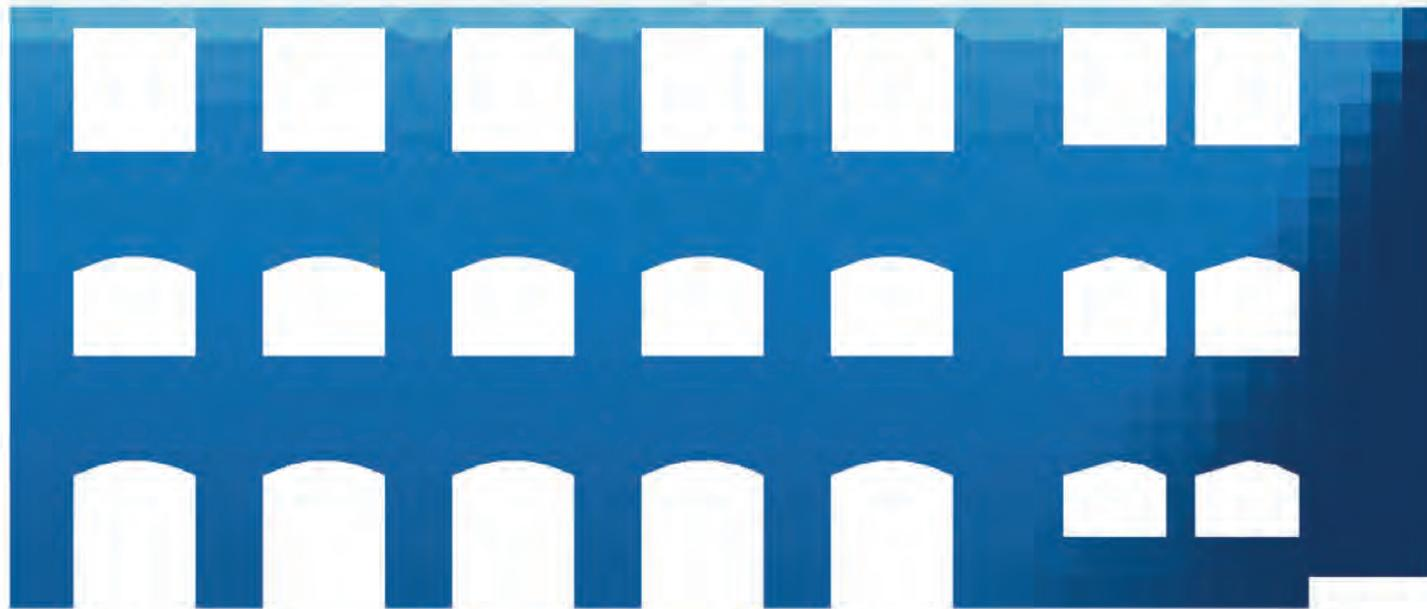
Some tools are built from scratch. When tools are not available elsewhere, we use existing research papers from various narrow fields and implement methods, algorithms, and procedures as code. Above is a tool that simulates annual driving rain on walls.
