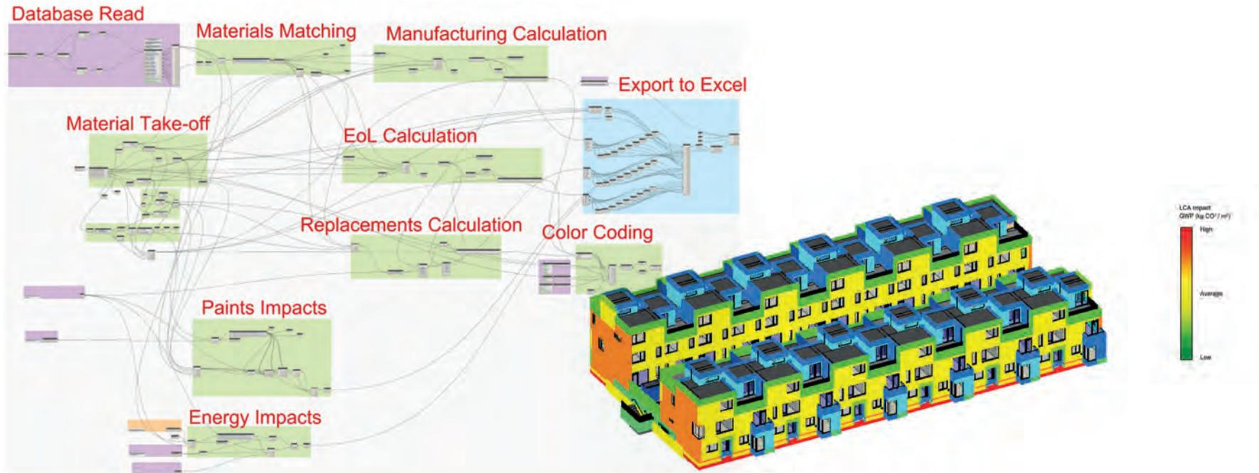
In this work, tools are built to couple logical processes and routines, and to bridge the existing simulation and calculation tools that are necessary to generate relevant feedback for the designers. Vandkunsten's project Havneviggen is analyzed with an LCA tool that utilizes the BIM7AA encoding system as well as the Ökobau LCA database.
