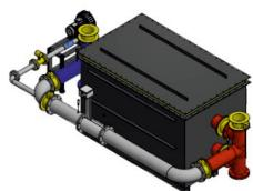
Figure 9. Photo and drawing of test facility for High Temperature Thermal Energy Storage at DTU. The facility contains a 1.5m<sup>3</sup> rock bed.
