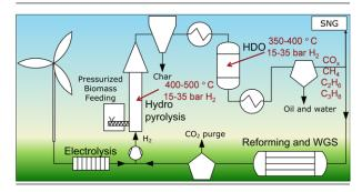
**Figure 1.** Schematic overview of a process for the catalytic hydropyrolysis of biomass to liquid fuel with downstream deep hydrodeoxygenation (HDO). Hydrogen may be derived from water electrolysis using surplus wind (or solar power, or by steam reforming of light pyrolysis gases). When hydrogen comes from wind or solar power, significant co-production of substitute natural gas (SNG) is possible.
