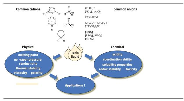
Figure 2. Ionic liquids ion pairs and tunable properties
