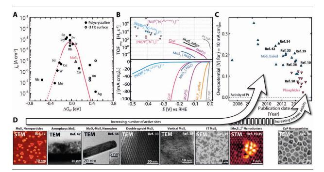
**Figure 7** displays (A) HER volcano plot for metals and MoS2 (B) TOF avg plots with linear sweep voltammograms of various HER catalysts. State-of-the-art Ni-based homogeneous catalysts are also included for comparison. (C) Chronological trend in overpotential of MoS2-based and phosphide HER catalysts. (D) Representative microscopy images of HER catalysts. Reproduced from [2]
