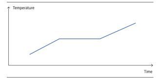
Figure 10. Development of temperature of aluminum upon heating with constant power input
