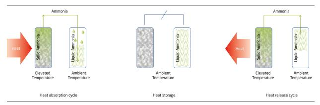
Figure 11. Principle of Thermo-Chemical Energy Storage illustrated by a system involving ab- and desorption of ammonia. Starting from the left, heat is added to the ammonia-containing compound, and ammonia is liberated. In the middle, a valve is closed to isolate the ammonia. To the right, the valve has been opened and the ammonia is allowed to react, release heat again and close the cycle. Figure by courtesy of D. Blanchard.
