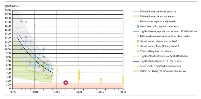
**Figure 7.** Price development for Li ion batteries for vehicles from [12]. Red circle shows the price of a Chevy Volt battery 2017 (145 \$/kWh).
