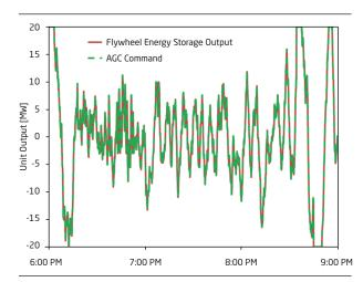
**Figure 3.** The reaction of a flywheel (MW input/output) in response to signals from the automatic generation control. It can be seen that, within the accuracy of the graph (note the axis scaling), the flywheel follows the signals completely. Source: Beacon Power.
