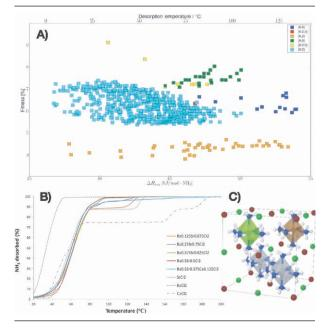
Figure 3. A) Predicted ammonia release (wt.%) within a temperature range relevant for automotive DeNOx for a class of novel binary and ternary metal halides for ammonia storage. Using genetic algorithms and DFT calculations, it was possible to identify the top 5-10 candidates by calculating only a few percent of >100.000 possible structures. B) Experimental confirmation of the predicted ammonia release conditions. C) The ternary metal halide ammine template crystal structure [28].
