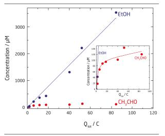
**Figure 5** displays the amount of ethanol and acetaldehyde produced over oxygen-derived copper in a 0.1M KOH at -0.33 V. Oxygen-derived copper is a copper surface which was first oxidized and then reduced leading to an increased surface area of roughly a factor fifty. Reproduced from [10]. The compound CH3CHO is acetaldehyde.
