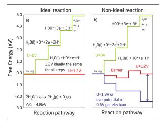
**Figure 3.** Schematic free energy diagram for water splitting. a) displays the ideal case where all intermediates are bond equally strong, while b) shows a more realistic case where an overpotential of 0.6 V occurs due to a too strong bonding of atomic oxygen. Reproduced from ref [6]).
