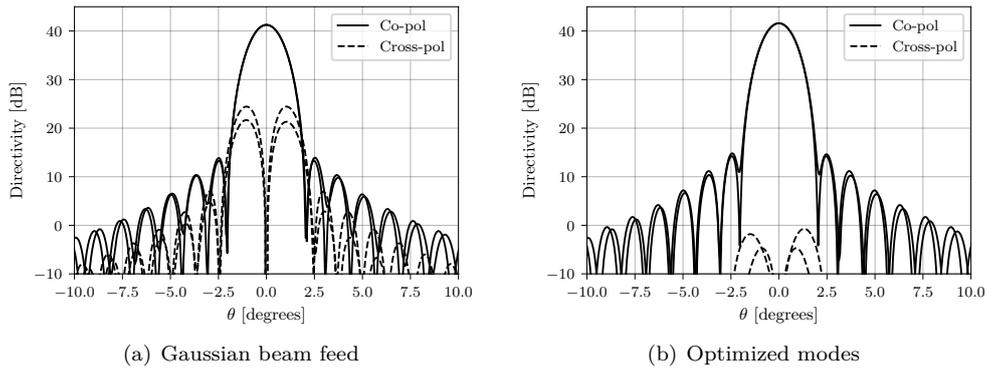
**Figure 3.5:** Validation of the aperture field optimization procedure. Secondary patterns of an  $f/D = 0.5$  reflector illuminated by modes dictated by the upper right plot of Figure 3.3 (PO+PTD calculation). The secondary pattern when the same reflector is illuminated by a perfectly co-polarized Gaussian beam is shown for reference. Asymmetry and diagonal plane cuts are plotted.
