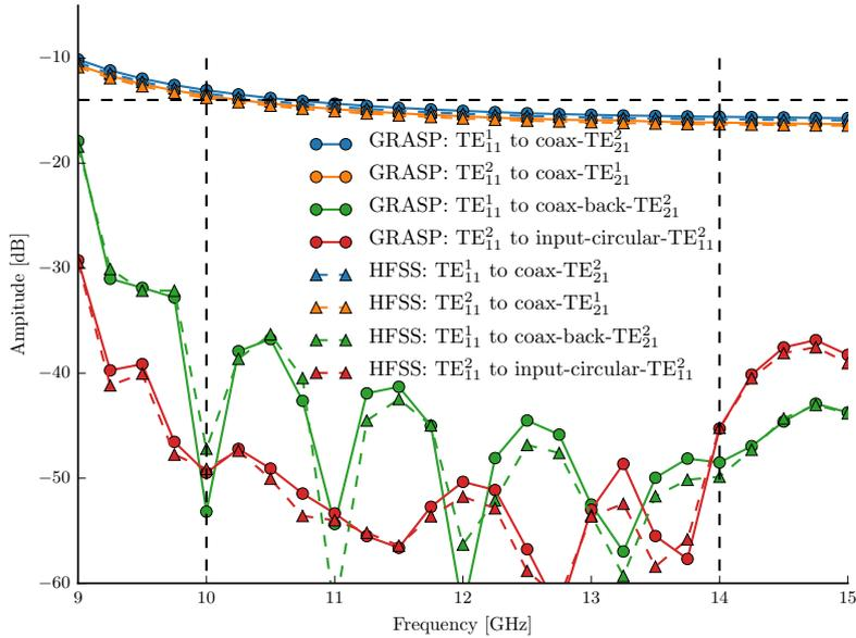
**Figure 5.8:** Computed scattering parameters compared with HFSS [94]. HFSS uses a volumetric finite element solver as opposed to the surface integral equation solver of GRASP. Markers indicate evaluated frequency points. Results calculated with GRASP are shown with full lines and circular markers, corresponding results calculated with HFSS have the same colors, but are shown with dashed lines and triangular markers.
