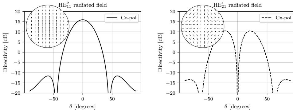
**Figure 6.3:** Radiation patterns of  $\text{HE}_{11}$  and  $\text{HE}_{21}$  hybrid modes from an impedance waveguide of radius  $a = 25$  mm with wall reactances  $x_z = -1$  and  $x_\phi = 1$ . The cut shown is  $\phi = 0^\circ$  where the  $\text{HE}_{21}$  mode is purely cross polarized. The  $\text{HE}_{11}$  radiates almost no cross polarization in any plane. The patterns are evaluated at 13 GHz and calculated from numerical integration of the aperture E- and H-fields in GRASP.
