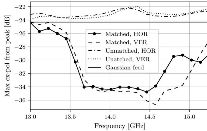
**Figure 5.14:** Maximum cross polarization within  $\theta \in [-1.5^\circ, 1.5^\circ]$  compared to peak co-polar directivity. The values for the horn without coupler and a perfectly polarized Gaussian beam feed are shown for reference.
