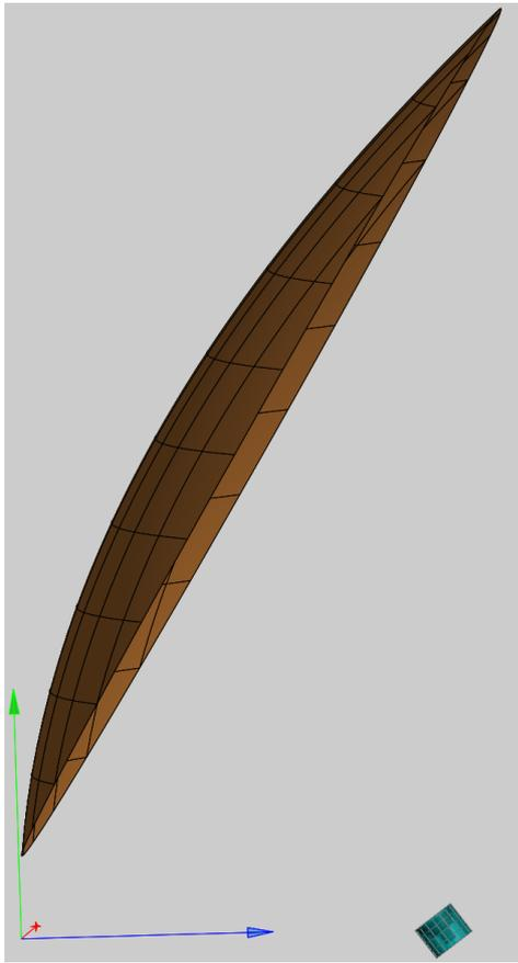
Fig. 4. Model of the entire antenna with  $f/D = 0.5$ .
