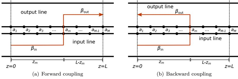
**Figure 5.1:** Coupling between two transmission lines at discrete coupling points. The two lines can represent two waveguides or two modes in the same waveguide.  $\beta_{\text{in}}$  and  $\beta_{\text{out}}$  are the phase constants of the input and output mode, respectively.  $a_1, a_2, \dots, a_M$  are coupling coefficients at  $M$  evenly spaced coupling points.  $L$  is the length of the coupler and  $z_m$  is the  $z$ -position of the  $m$ th coupling point.
