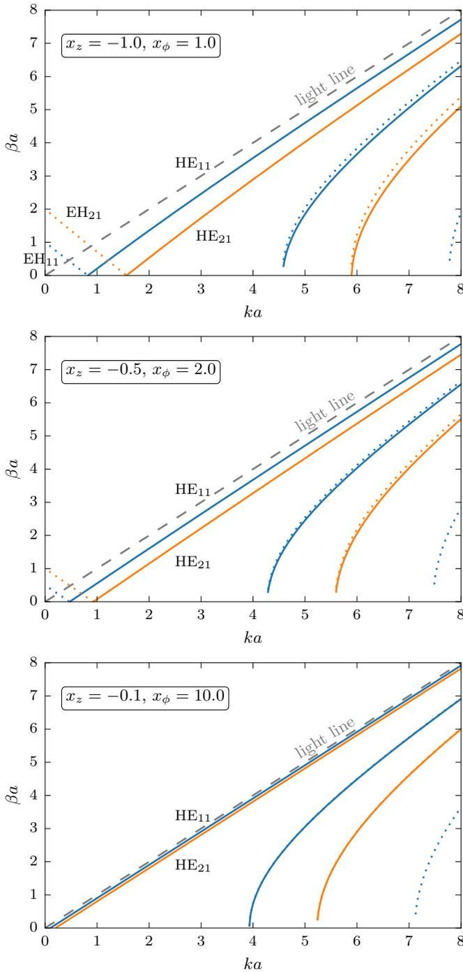
Fig. 2. Dispersion diagrams for a circular waveguide with three sets of surface reactances fulfilling the balanced hybrid condition:  $x_z x_\phi = -1$ . Blue curves represent  $m = 1$  azimuthal variation and orange curves represent  $m = 2$  variation. Full lines are HE modes and dotted lines are EH modes.
