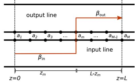
Fig. 2. Loose coupling with discrete coupling points.
