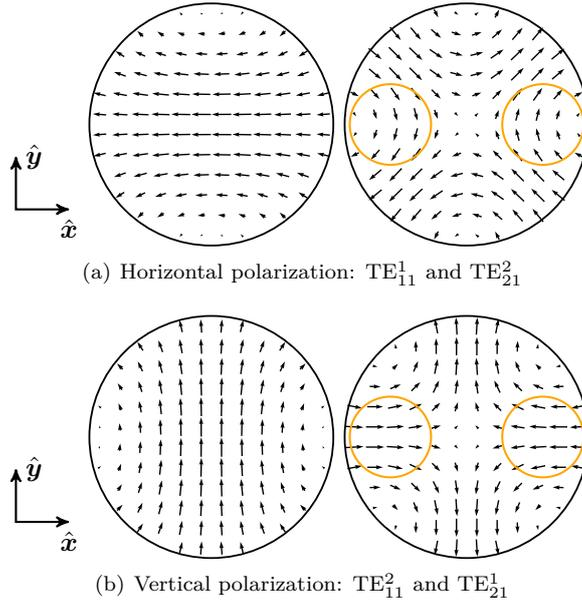
**Figure 2.8:** Transverse fields of the  $TE_{21}$  modes needed for matched feed operation shown together with the corresponding  $TE_{11}$  mode for each polarization. The desired regions of cross-polar field are highlighted. A  $y$ -offset reflector is assumed. The  $TM_{11}$  modes are omitted here.
