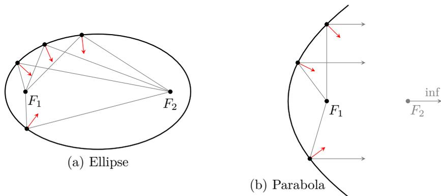
**Figure 2.1:** Focusing properties of ellipses and parabolas. The parabola is a special case of the ellipse, where one of the foci is in infinity, and it is therefore well suited for sending radio signals *far away*. Red arrows indicate normal vectors.
