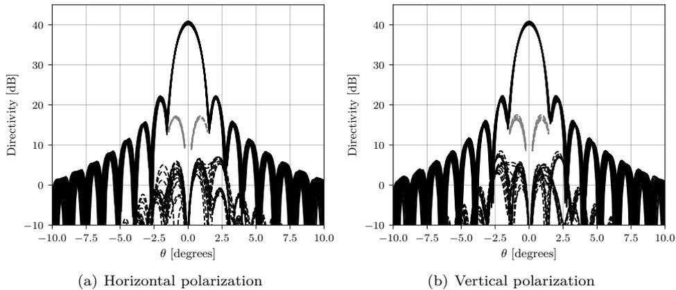
**Figure 5.15:** Secondary patterns of the reflector with the optimized horn.  $0^\circ$ ,  $45^\circ$ , and  $90^\circ$  cuts are plotted for nine frequencies across the band 13.75 GHz to 14.5 GHz. Co-polar radiation is in full lines, cross-polar is in dashed lines. The cross polarization of the system with an unmatched feed is indicated in dashed grey within the  $\theta \in [-1.5^\circ, 1.5^\circ]$  range.
