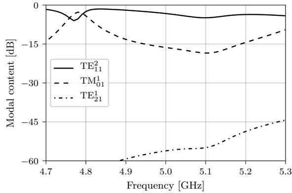
**Figure A.4:** Mode content in the aperture of the matched feed when excited by the TE<sub>11</sub><sup>2</sup> mode ( $y$ -polarized).
