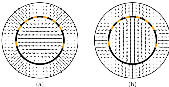
**Figure 5.5:** Modal E-fields of the incident circular and desired coaxial modes for the two polarizations: (a)  $TE_{11}^1$  to  $TE_{21}^2$  and (b)  $TE_{11}^2$  to  $TE_{21}^1$ . The azimuthal positions of the coupling holes are indicated in orange:  $\phi = \{30.9^\circ, 53.8^\circ, 76.7^\circ, 102.1^\circ, 125.0^\circ, 147.9^\circ, 187.6^\circ, 347.4^\circ\}$ .
