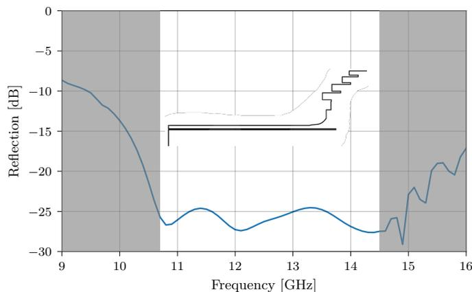
**Figure 5.11:** Reflection from the coaxial input with an axially corrugated horn. Transition and first corrugations optimized for low reflection. The unshaded area is the frequency interval of interest. The generating curve of the circular symmetric horn is shown in the inset.
