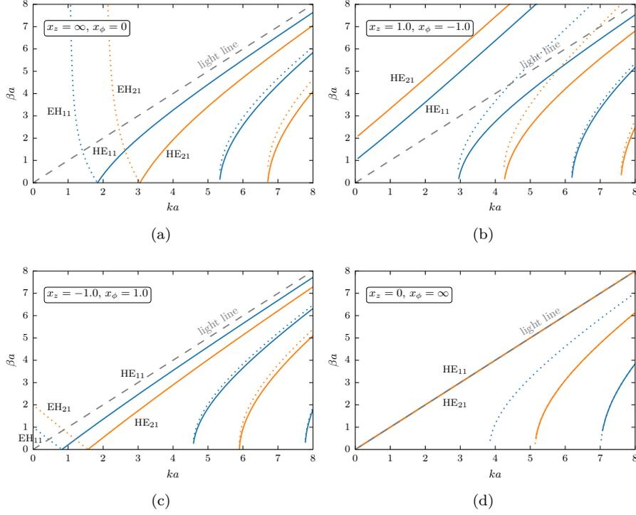
**Figure 6.1:** Dispersion diagrams for different balanced surface impedances, i.e.  $x_z x_\phi = -1$ . Blue curves are  $m = 1$  modes and orange curves are  $m = 2$  modes. Stars correspond to balanced EH modes ( $\gamma = -1$ ) and dots to balanced HE modes ( $\gamma = 1$ ).
