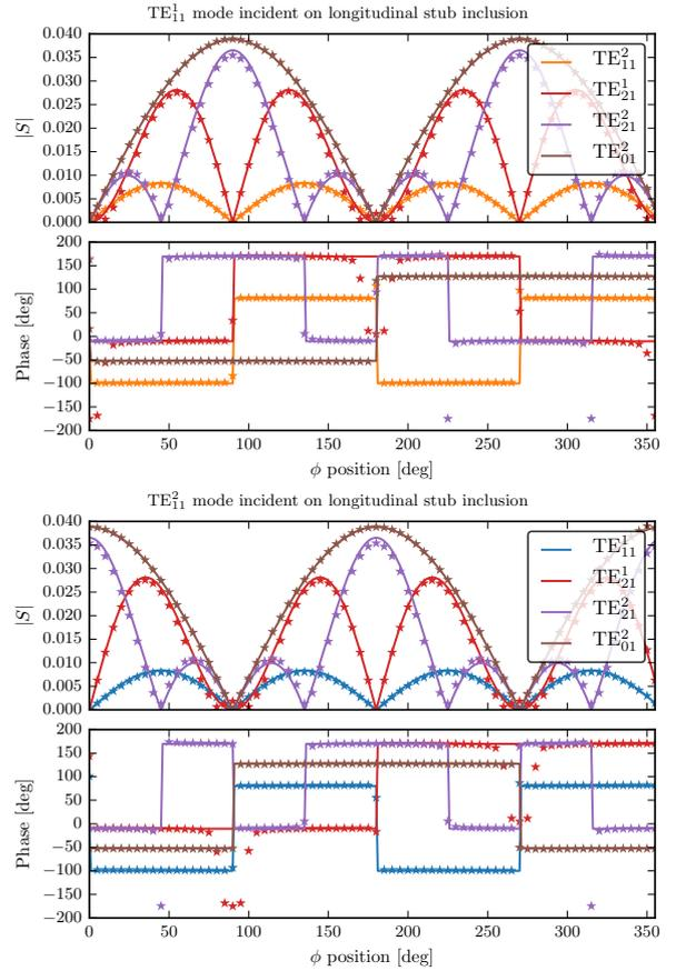
Fig. 2. Modes generated by longitudinal stub versus stub azimuthal position for  $x$ -polarized (top) and  $y$ -polarized (bottom)  $TE_{11}$  incidence. Solid lines are calculations from the simple model and the stars are full wave MoM simulations from GRASP.
