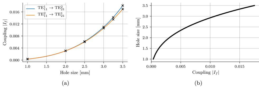
**Figure 5.6:** Coupling of desired modes in a single coaxial slice with the azimuthal hole distribution shown in Figure 5.5. The waveguide dimensions are listed in Figure 5.2(a). (a) Shows the relationship between hole size and coupling values. The markers show simulated hole sizes and cubic splines interpolate between. The coupling value for each size is an average over the design frequency band. (b) Shows the inverse of the average of the two curves in (a).
