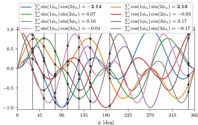
**Figure 5.4:**  $TE_{11}$  to  $TE_{21}$  and  $TE_{31}$  mode coupling in circular or coaxial waveguide geometries. Each line represents the coupling from one of the input mode polarizations to an output mode. Each inclusion is represented by a vertical line and can contribute coupling to several modes (dots). The total coupling of the input-output mode pairs is summed and shown in the legend.
