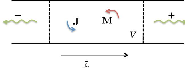
**Figure 4.1:** Electric and magnetic currents,  $\mathbf{J}$  and  $\mathbf{M}$ , exciting modes in a waveguide.
