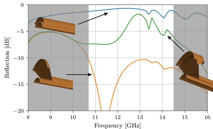
**Figure 5.10:** Reflections of a coaxial waveguide: with no alterations (blue), with a simple flare (orange), and with a flare and an axial corrugation (green). The inset figures show a quarter of the rotationally symmetric devices. The inner coaxial radius is 11.1 mm and the outer is 13.6 mm. The unshaded area is the frequency interval of interest.
