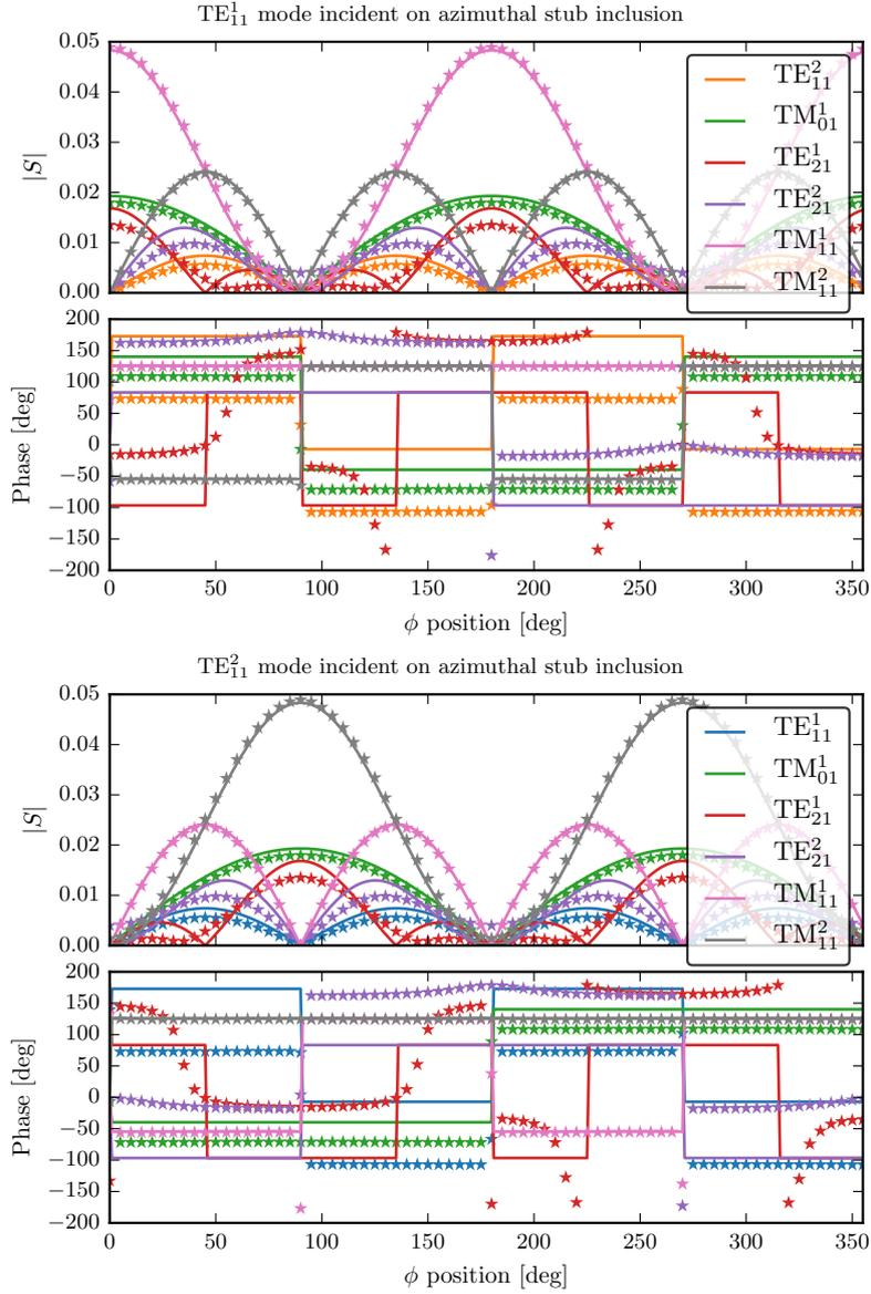
**Figure 4.7:** Mode generation from azimuthal stub as function of stub  $\phi$ -position around the waveguide wall. The incident mode is the TE<sub>11</sub> mode of set 1 (top) and set 2 (bottom). Full lines are the analytical model and stars are from MoM simulations in GRASP.
