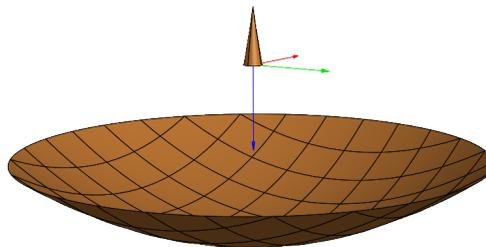
**Figure 2.2:** Simplest rotationally symmetric reflector antenna system: paraboloidal reflector and feed pointed toward vertex. A real antenna would require support structures for the feed.
