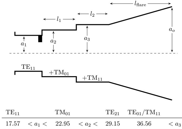
**Figure A.1:** Topology of the  $TM_{01}$  matched feed. Below it, the cutoff radii in mm of waveguide modes in a circular waveguide at 5 GHz are listed. The proper intervals of the horn sections are indicated.
