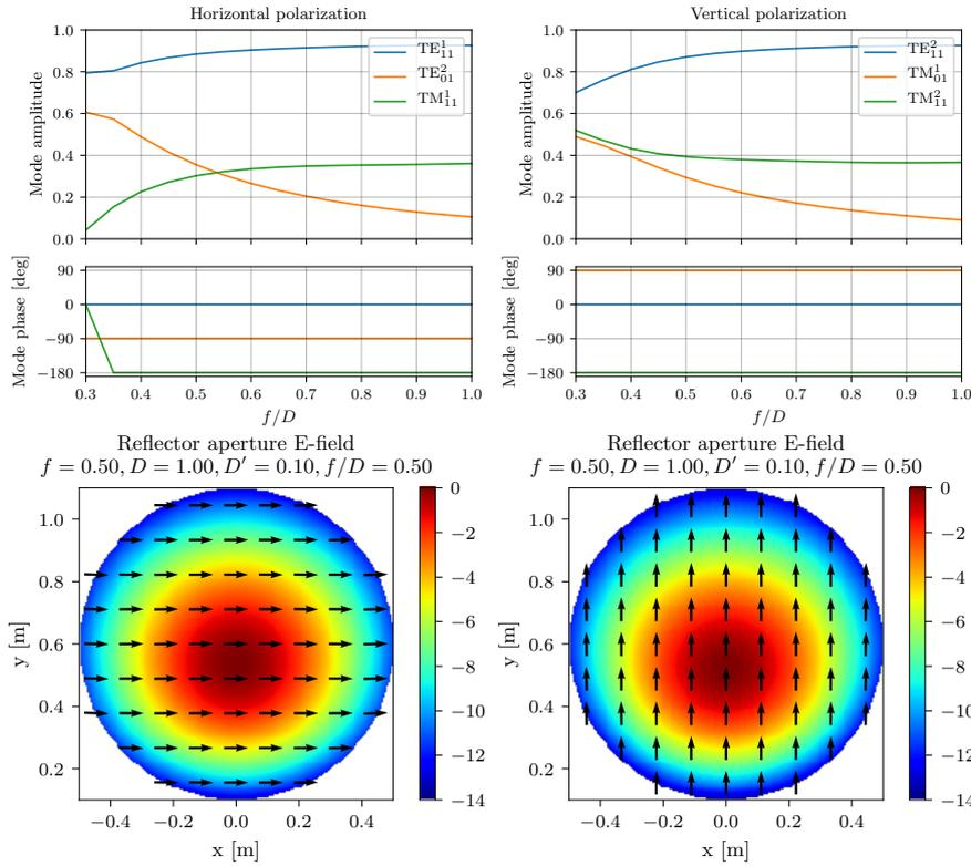
**Figure 3.4:** Optimized mode excitation coefficients for  $f/D$  values between 0.3 and 1.  $TE_{21}$  modes have been excluded. Resulting reflector aperture fields for  $f/D = 0.5$  are shown.  $K_{cr} = 50$ .
