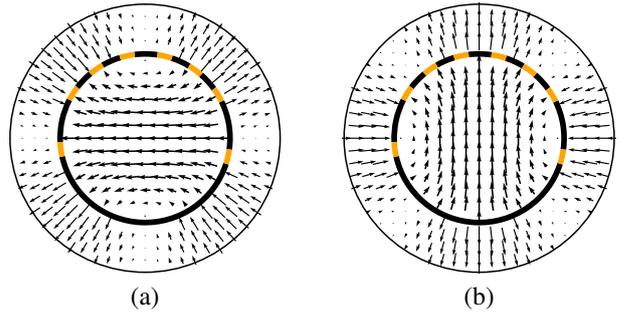
Fig. 3. Modal E-fields of the incident circular and desired coaxial modes for the two polarizations: (a)  $TE_{11}^1$  to  $TE_{21}^2$  and (b)  $TE_{11}^2$  to  $TE_{21}^1$ . The coupling holes are indicated in orange and their angular positions in degrees are  $\phi = \{30.9^\circ, 53.8^\circ, 76.7^\circ, 102.1^\circ, 125.0^\circ, 147.9^\circ, 187.6^\circ, 347.4^\circ\}$ .
