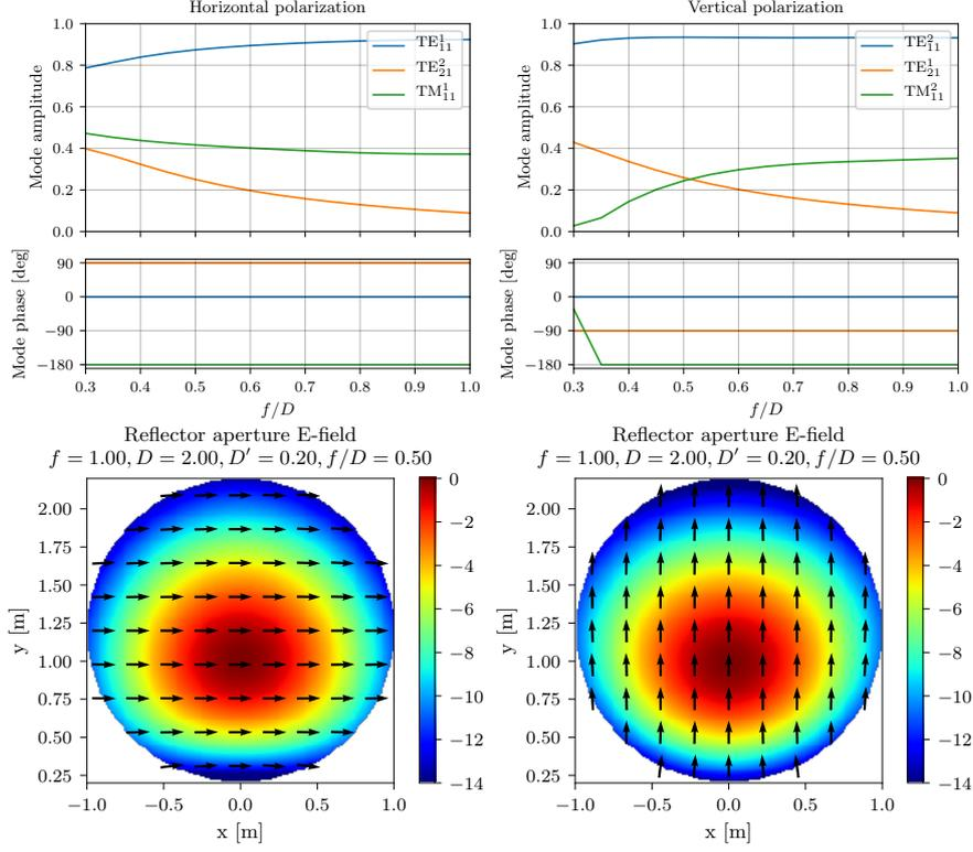
**Figure 3.1:** Optimized mode excitation coefficients for  $f/D$  values between 0.3 and 1. Zero-order modes have been excluded. Resulting reflector aperture fields for  $f/D = 0.5$  are shown.  $K_{cr} = 50$ .
