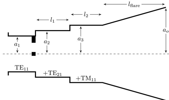
**Figure 2.7:** Topology of the matched feed horn presented by Rudge and Adatia [6] and most other designs in the literature. Only  $TE_{11}$  can propagate where the radius is  $a_1$ ,  $TE_{21}$  and  $TM_{11}$  are excited in subsequent sections. The inclusions at the  $a_1$  to  $a_2$  step represent the asymmetric mode launcher.
