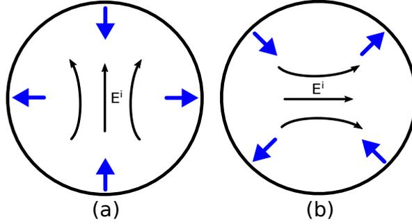
**Figure 4.3:** Azimuthal positions of radial currents to excite maximum  $TE_{21}$  mode of (a): set 1, and (b): set 2. Arrows indicate the mutual directions the currents must have to add constructively to the  $TE_{21}$  modes. Blue arrows indicate electric current. The incident  $TE_{11}$  modes from which the currents need to be excited are indicated with black arrows.
