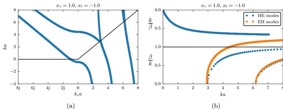
**Figure B.1:** Waveguide with wall impedances  $Z_z = Z_0 j$ ,  $Z_\phi = -Z_0 j$ . (a):  $k$  values found from a list of  $k_c$  values. Only points above the black line are usable. (b): Dispersion plot from accepted  $(k, k_c)$  pairs. Here the black line is the light line.
