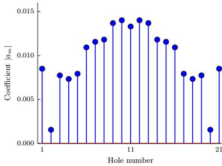
Fig. 5. Optimal coupling coefficients minimizing the maximum deviation from the desired coupling in both bands, i.e.  $-14$  dB in the passband and  $-\infty$  dB in the stopband. All coefficients have the same phase.
