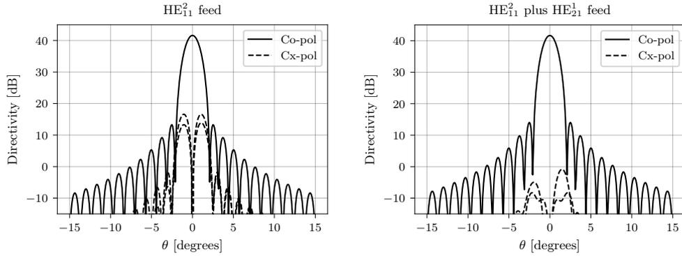
**Figure 6.4:**  $yz$ -offset reflector system with  $f/D = 0.8$  illuminated by the hybrid modes of Figure 6.3. The left plot is of pure  $\text{HE}_{11}$  illumination, i.e. virtually zero cross polarization of the feed. The right plot shows how the feed tilt can be compensated by addition of  $-18.5$  dB  $\text{HE}_{21}$  in phase quadrature. The cross polarization is shown in both  $\phi = 0^\circ$  and  $\phi = 45^\circ$
