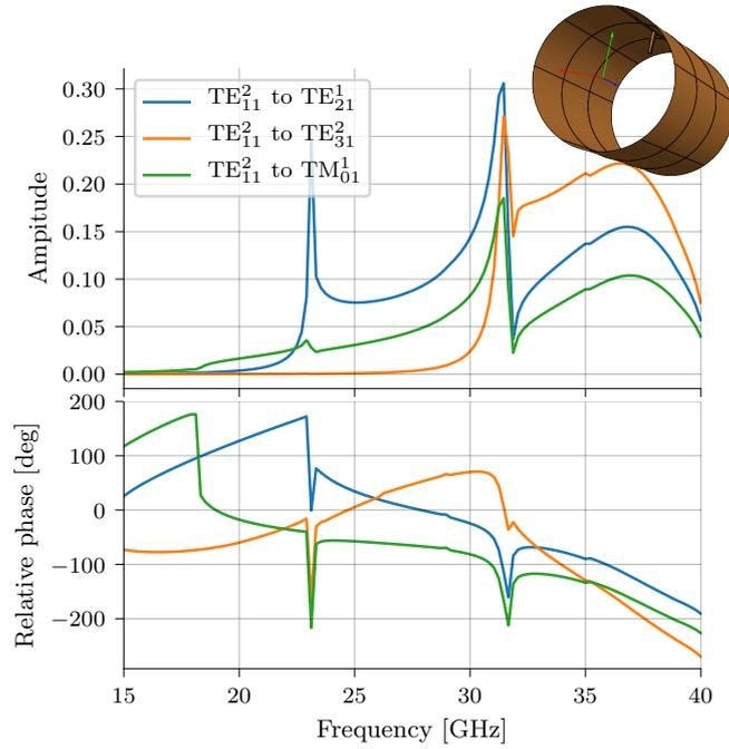
(a) radial pin at  $\phi = 90^\circ$
