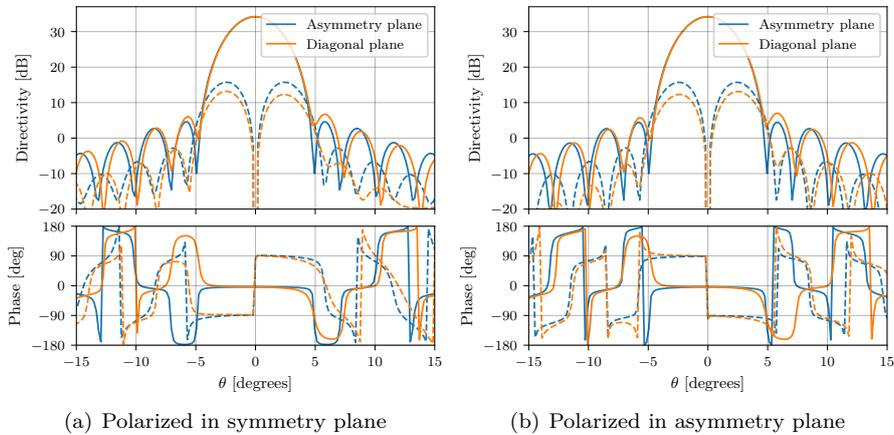
**Figure 2.5:** Radiation pattern of offset reflector antenna defined in Table 2.1 [3] illuminated by a purely co-polarized Gaussian beam feed. Cuts in the asymmetry and diagonal planes are shown, there is no cross polarization in the symmetry plane. Cross polarization patterns are drawn with dashed lines. Reflector scattering is calculated with PO+PTD in GRASP.
