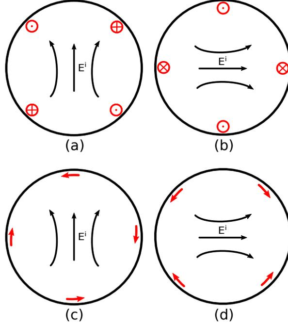
**Figure 4.4:** Azimuthal positions of magnetic currents to excite maximum  $TE_{21}$  mode of (a) and (c): set 1, (b) and (d) : set 2. Arrows indicate the mutual directions the currents must have to add constructively to the  $TE_{21}$  modes. Red arrows indicate magnetic current. The incident  $TE_{11}$  mode from which the currents need to be excited in each case is indicated with black arrows.
