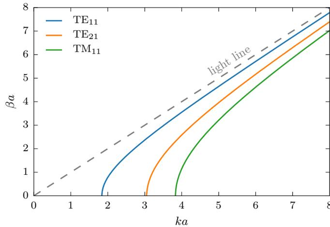
**Figure 2.9:** Dispersion plot of selected modes in a circular waveguide.  $k = \frac{2\pi f}{c}$  is the free space wavenumber.  $\beta = \sqrt{k^2 - k_c^2}$  is the propagation constant of the mode, with  $k_c$  being the smallest wavenumber at which the mode can propagate.  $a$  is the radius of the waveguide.
