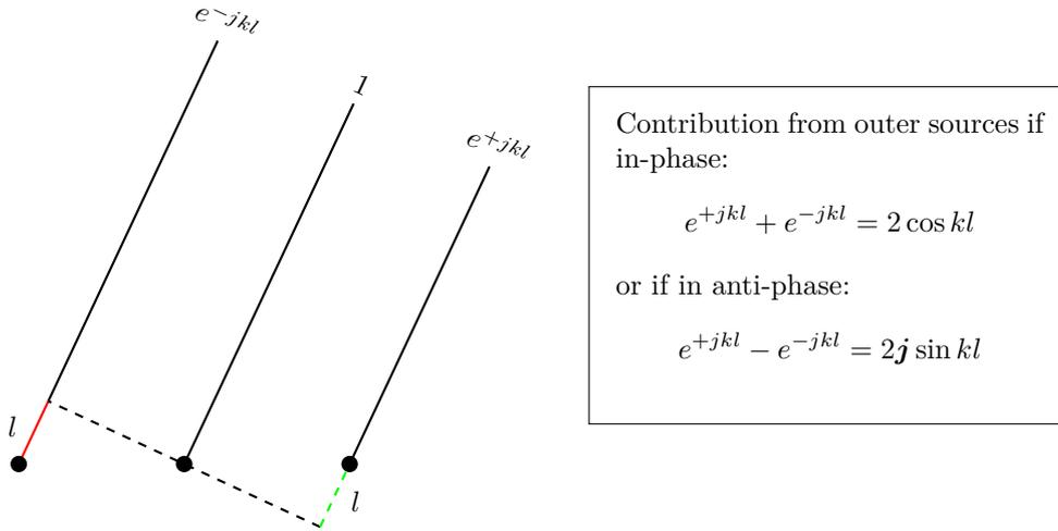
**Figure 2.6:** Radiation from displaced sources. If the outer elements are in phase with the middle element, their contribution will be in phase with the middle one's and maximum at boresight. If one of the outer elements is in phase with the middle element and the other in anti-phase, their contribution will be in phase quadrature with the middle one's and maximum when  $kl = \frac{\pi}{2}$ .
