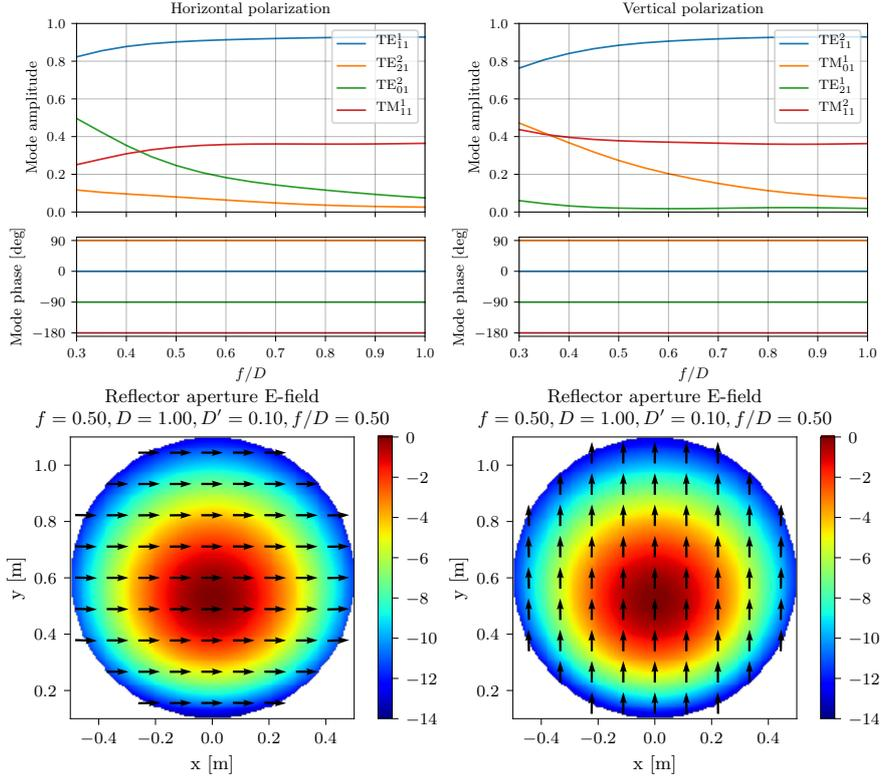
**Figure 3.3:** Optimized mode excitation coefficients for  $f/D$  values between 0.3 and 1. Horizontal (left column) and vertical (right column) polarization. Resulting reflector aperture fields for  $f/D = 0.5$  are shown.  $K_{cr} = 50$ .
