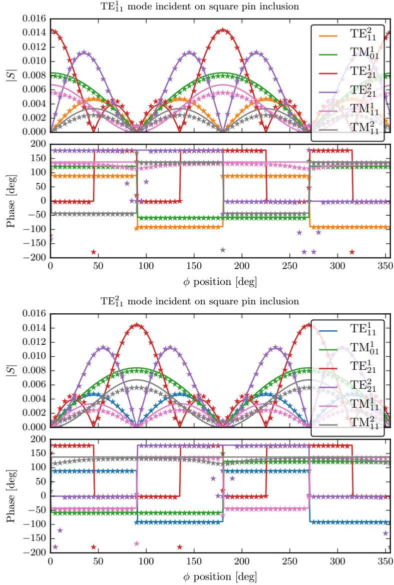
**Figure 4.6:** Mode generation from radial pin as function of pin  $\phi$ -position around the waveguide wall. The incident mode is the TE<sub>11</sub> mode of set 1 (top) and set 2 (bottom). Full lines are the analytical model and stars are from MoM simulations in GRASP.
