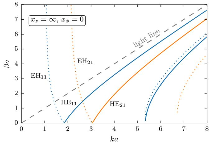
Fig. 1. Dispersion diagram for a circular waveguide with infinite longitudinal impedance,  $x_z = \infty$  and zero azimuthal,  $x_\phi = 0$ . This corresponds to a corrugated surface where the corrugations are  $\lambda/4$  deep. Blue curves represent  $m = 1$  azimuthal variation and orange curves represent  $m = 2$  variation. Full lines are HE modes and dotted lines are EH modes.
