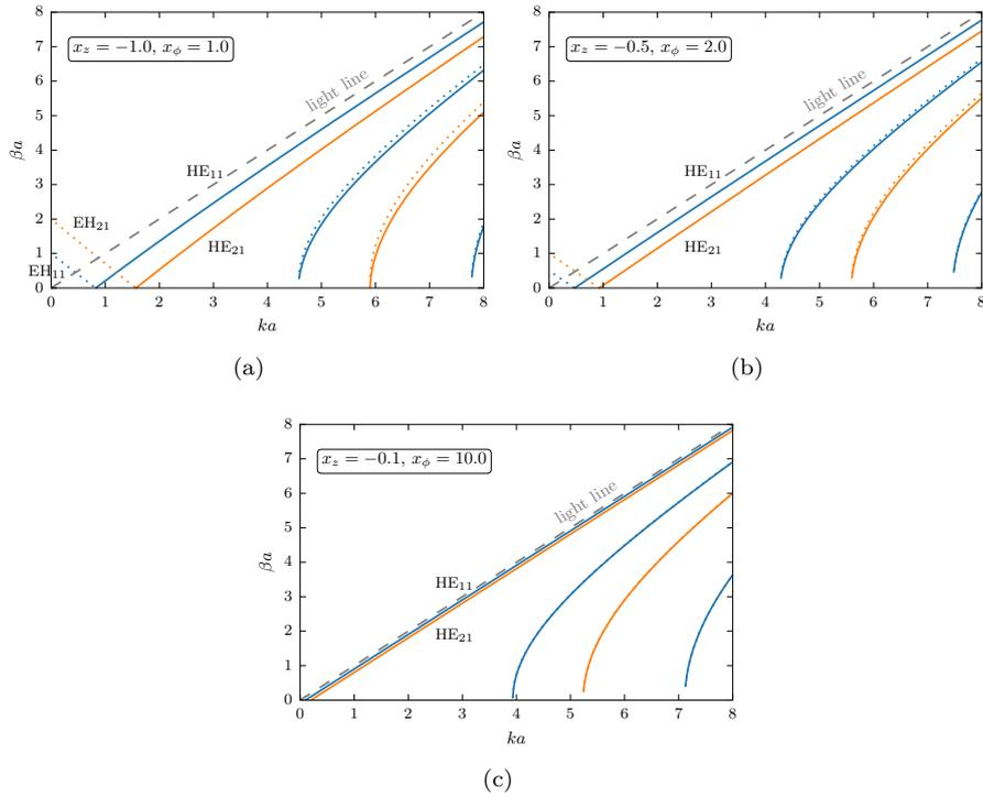
**Figure 6.2:** Dispersion plots for different balanced surface impedances, i.e.  $x_z x_\phi = -1$ . All four cases are with a capacitive reactance in the  $z$ -direction and thus an inductive reactance in the  $\phi$ -direction. Blue curves are  $m = 1$  modes and orange curves are  $m = 2$  modes. Dotted lines correspond to balanced EH modes ( $\gamma = -1$ ) and full lines to balanced HE modes ( $\gamma = 1$ ).
