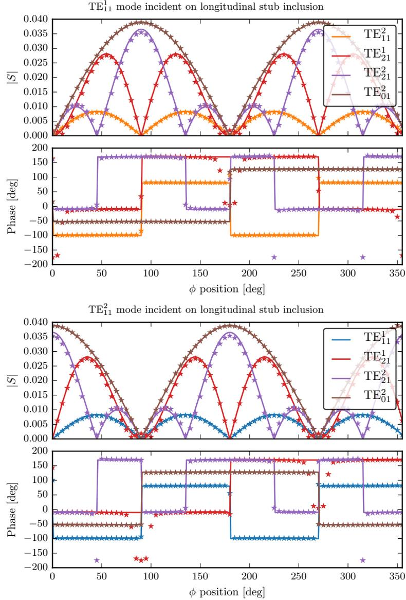
**Figure 4.5:** Mode generation from a longitudinal stub as function of stub  $\phi$ -position around the waveguide wall. The incident mode is the  $\text{TE}_{11}$  mode of set 1 (top) and set 2 (bottom). Full lines are the analytical model and stars are from MoM simulations in GRASP.
