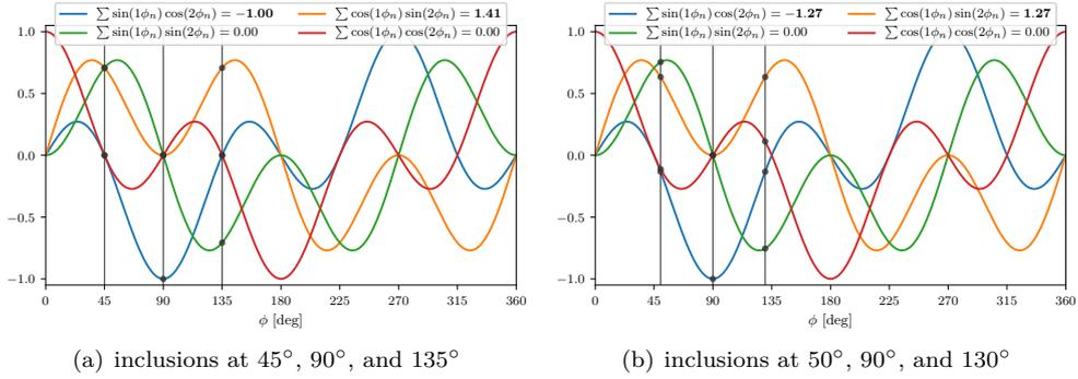
**Figure 5.3:**  $\text{TE}_{11}$  to  $\text{TE}_{21}$  mode coupling in circular or coaxial waveguide geometries. Each line represents the coupling from one of the input mode polarizations to an output mode. Each inclusion is represented by a vertical line and can contribute coupling to several modes (dots). The total coupling of the input-output mode pairs is summed and shown in the legend.
