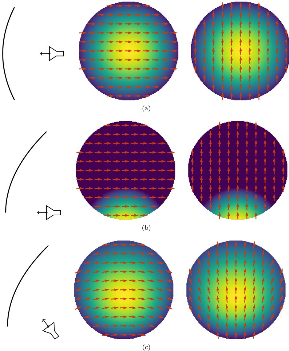
**Figure 2.4:** Symmetric and offset reflectors illuminated by Gaussian beam feeds with no cross polarization. Horizontally and vertically polarized reflector aperture fields are plotted for symmetric (a), offset with no feed tilt (b), and offset with feed tilt (c). The reflector  $f/D = 0.5$  in all three cases and the feed tilt is  $62^\circ$  in (c). It is evident that the cross polarization arises from the feed tilt.
