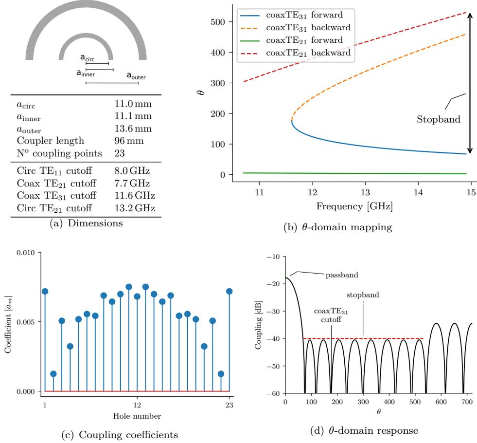
**Figure 5.2:** Design of directional coupler based on wanted and unwanted mode cutoffs (a). Phase constants are mapped to the  $\theta$ -domain (b) and optimal filter coefficients are found (c). The resulting response of the coupler is shown in (d).
