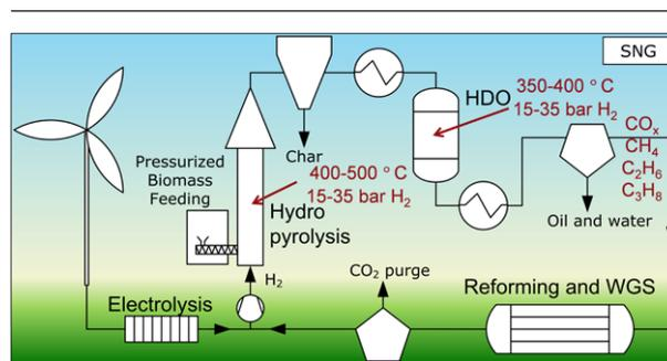
**Figure 1.** Schematic overview of a process for the catalytic hydropyrolysis of biomass to liquid fuel with downstream deep hydrodeoxygenation (HDO). Hydrogen may be derived from water electrolysis using surplus wind (or solar power, or by steam reforming of light pyrolysis gases). When hydrogen comes from wind or solar power, significant co-production of substitute natural gas (SNG) is possible.
