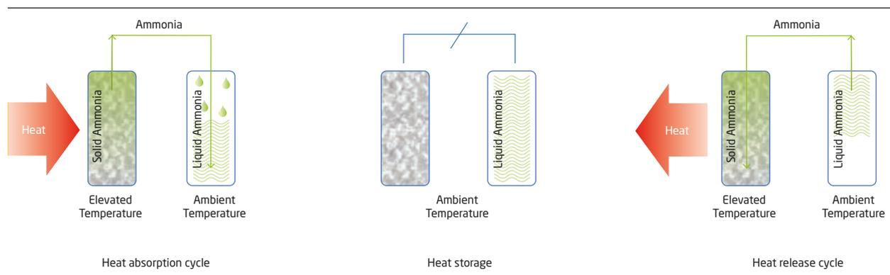
**Figure 11.** Principle of Thermo-Chemical Energy Storage illustrated by a system involving ab- and desorption of ammonia. Starting from the left, heat is added to the ammonia-containing compound, and ammonia is liberated. In the middle, a valve is closed to isolate the ammonia. To the right, the valve has been opened and the ammonia is allowed to react, release heat again and close the cycle. Figure by courtesy of D. Blanchard.
