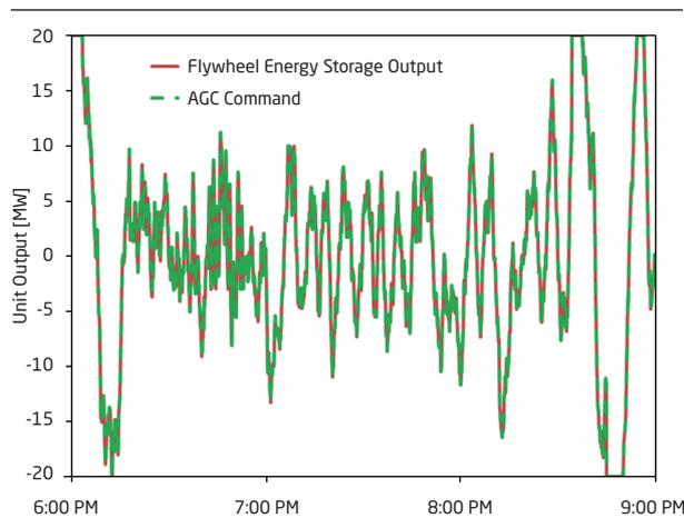
**Figure 3.** The reaction of a flywheel (MW input/output) in response to signals from the automatic generation control. It can be seen that, within the accuracy of the graph (note the axis scaling), the flywheel follows the signals completely. Source: Beacon Power.
