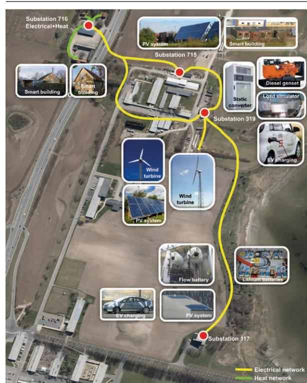
Figure 5. The importance of being able to test microgrid solutions under real or semi-real conditions, as in DTU's SYSLAB experimental research facility (illustration: DTU 2018).
