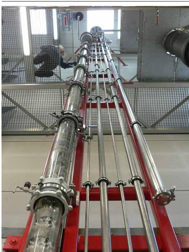
Figure 1. A view of the DTU absorption column
