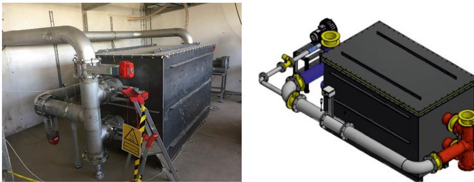
Figure 9. Photo and drawing of test facility for High Temperature Thermal Energy Storage at DTU. The facility contains a 1.5m<sup>3</sup> rock bed.
