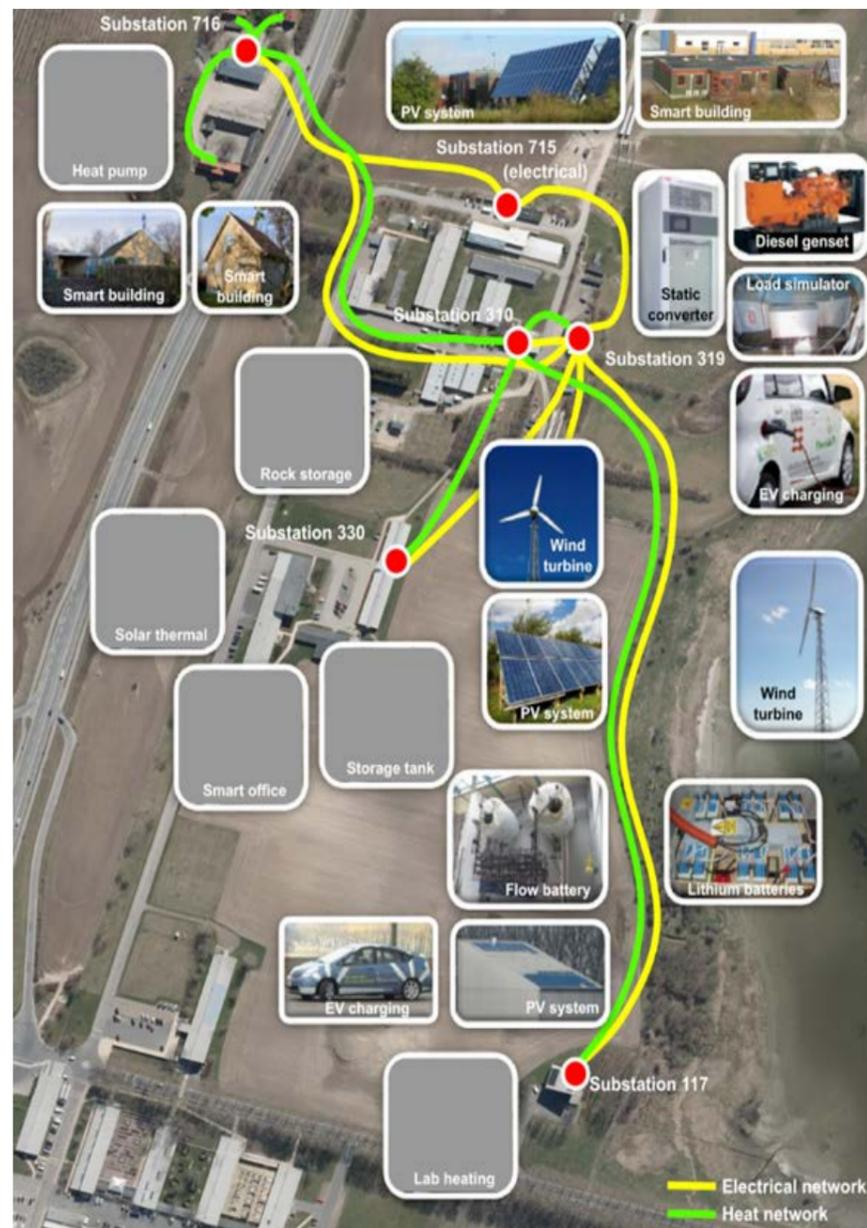
Figure 5. Lay-out and details of PowerLabDK/SYSLAB
