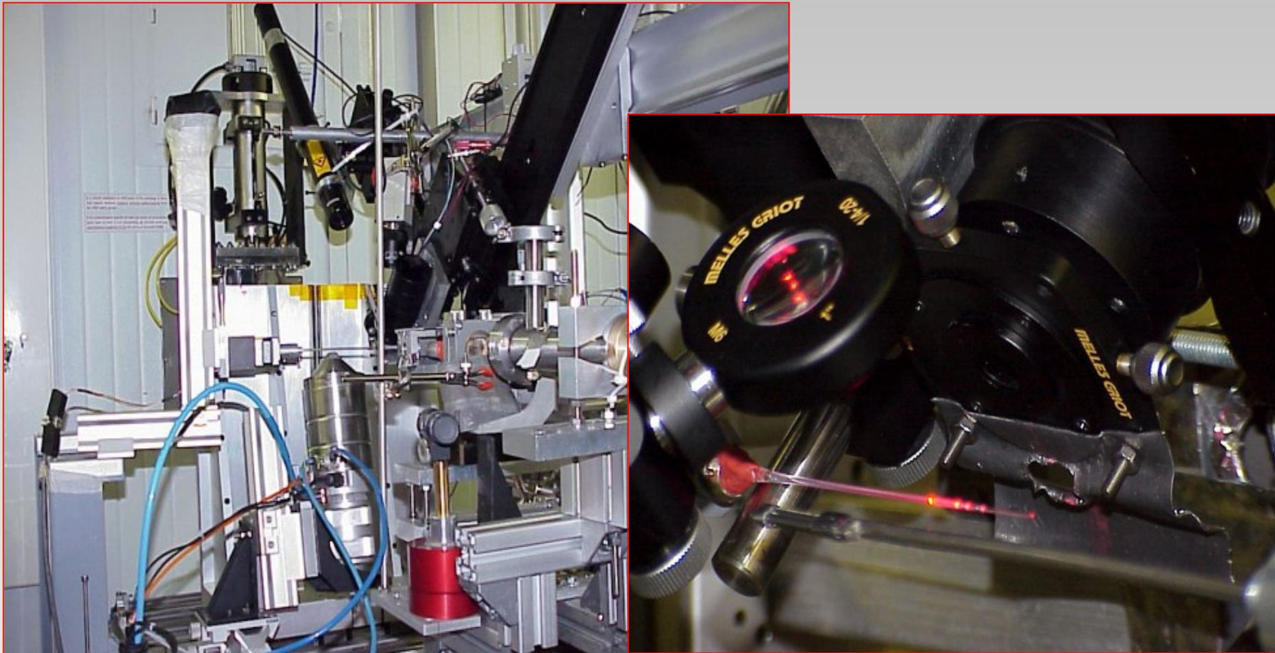
Example of a combined XRD/SAXS/DLS *in situ* experiment of zeolite synthesis
