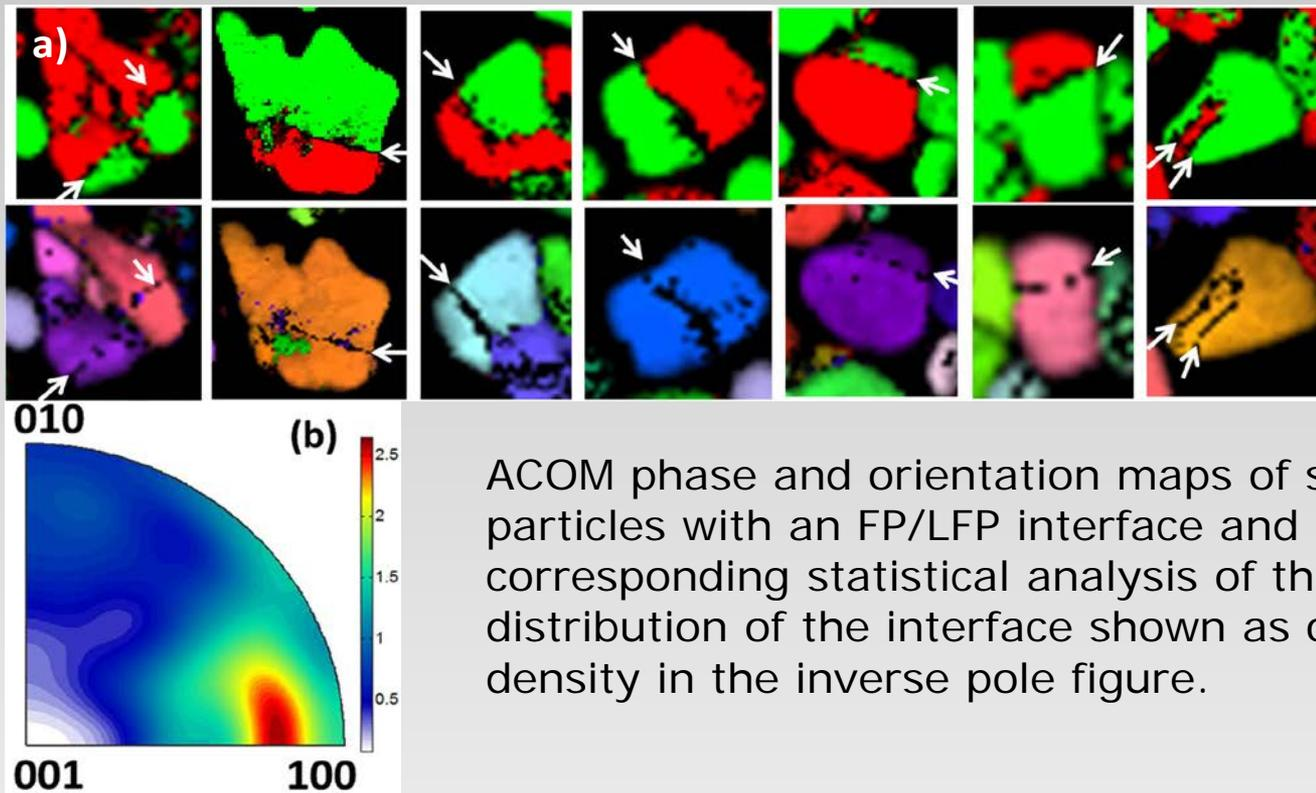
ACOM phase and orientation maps of single crystalline particles with an FP/LFP interface and the corresponding statistical analysis of the orientation distribution of the interface shown as orientation density in the inverse pole figure.
