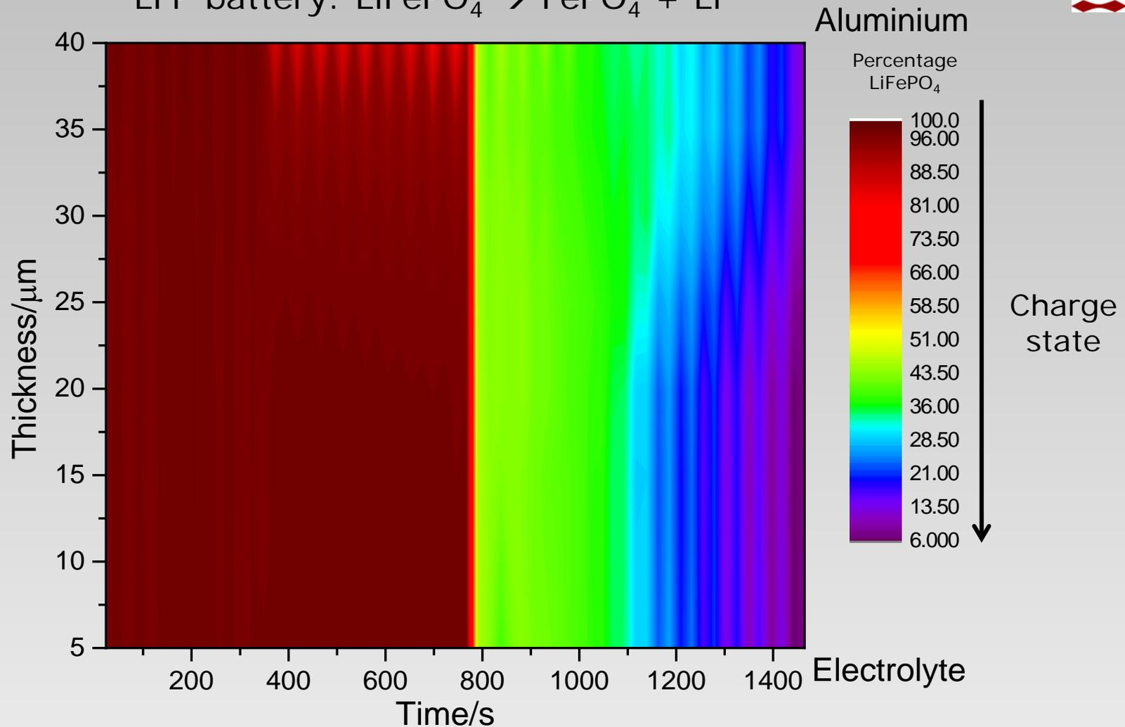
Gradient development during fast charge of  $\text{LiFePO}_4$  battery cell determined by Rietveld refinement
