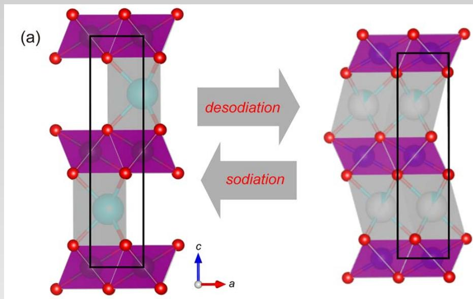
Crystal structures of the P2 and O2 phases
