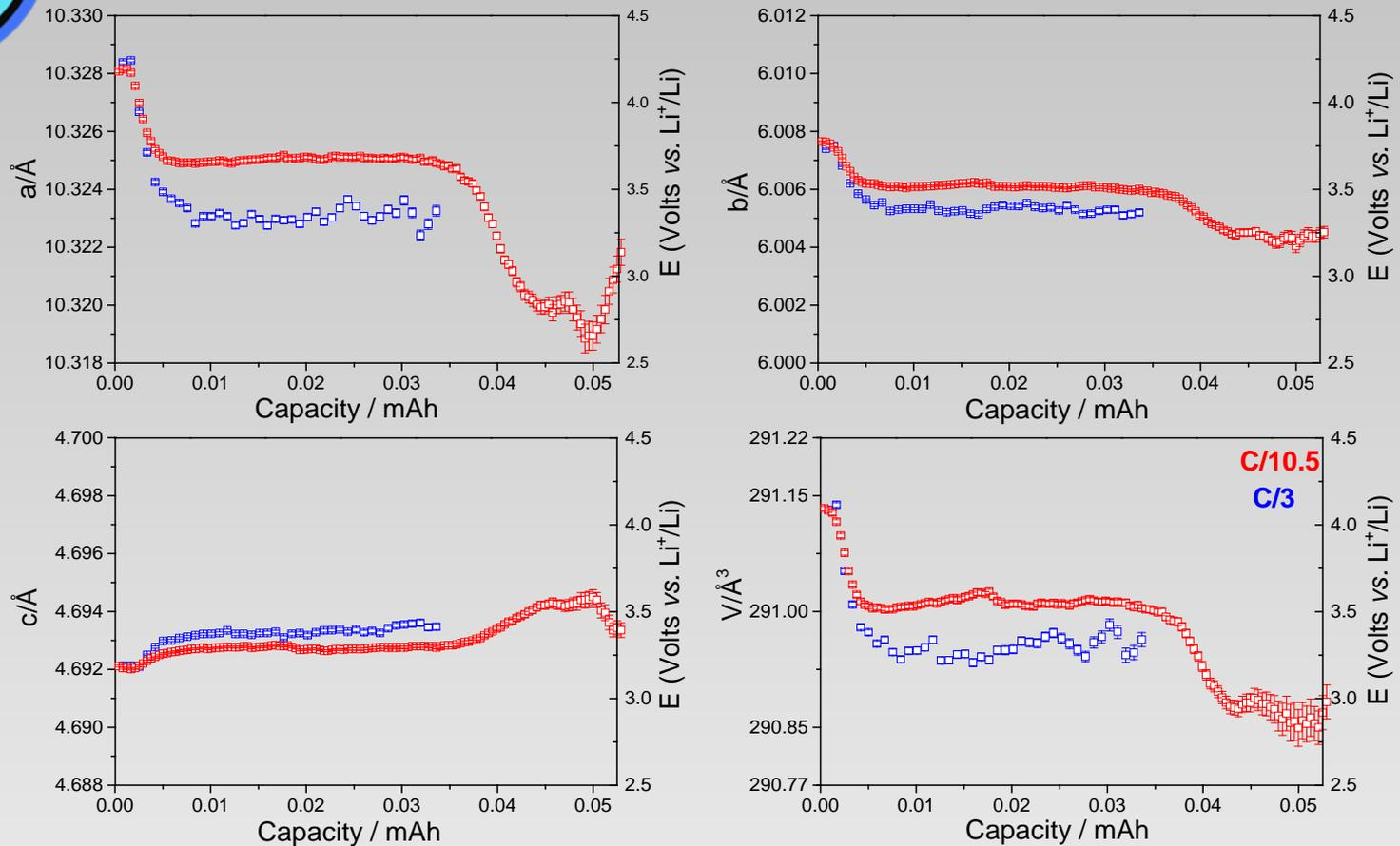
Unit cell variation for  $\text{LiFePO}_4$  during charging by C/10 and C/3.
