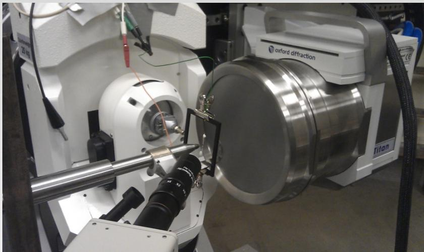
The capillary battery cell at beamline I711, Maxlab
