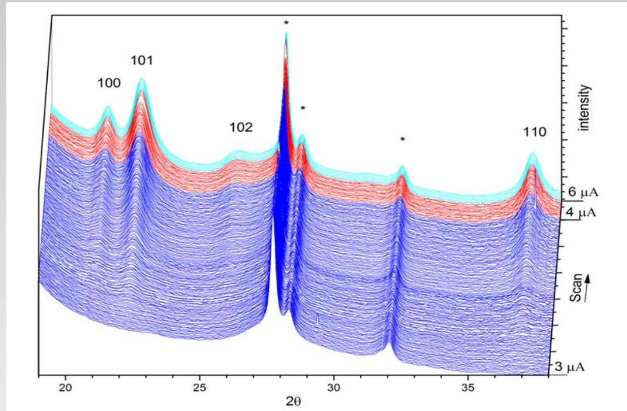
Lithium peroxide formation in a lithium-air ( $O_2$ ) battery during discharge
