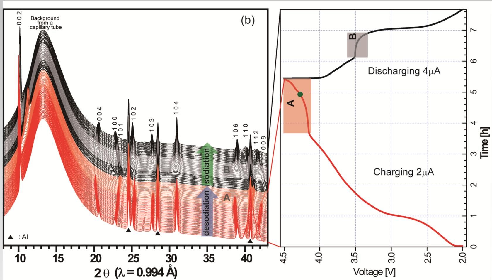
*In situ* synchrotron XRD patterns of the P2-Na<sub>0.7</sub>Fe<sub>0.4</sub>Mn<sub>0.4</sub>Co<sub>0.2</sub>O<sub>2</sub> electrode while a sodium ion battery capillary cell was charged at a current of 2  $\mu$ A to 4.5 V and discharged at a current of 4  $\mu$ A to 2.0 V.
