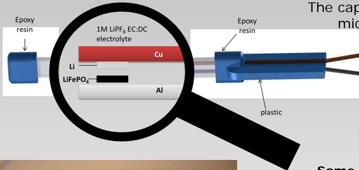
The capillary based *in situ* micro battery cell
