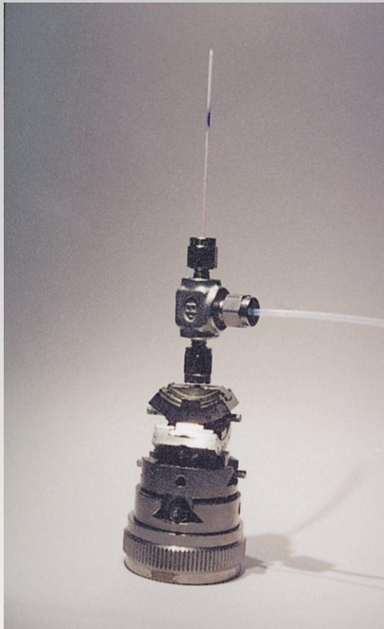
Capillary based Micro Reaction Cell
