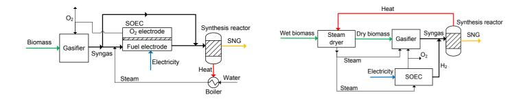
Figure 4. Right: wet biomass to SNG by integration of steam drying, gasification and SOEC. Left: dry biomass to SNG by gasification coupled with pressurized SOEC with internal methanation
