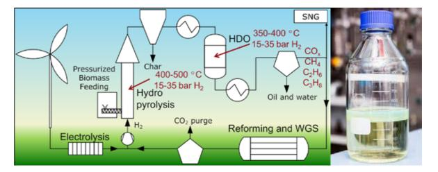
Figure 7. Proposed catalytic hydropyrolysis process diagram and example of hydropylrolysis liquids formed in the laboratory of DTU Chemical Engineering, showing the phase separation of oil (top) and water (bottom).
