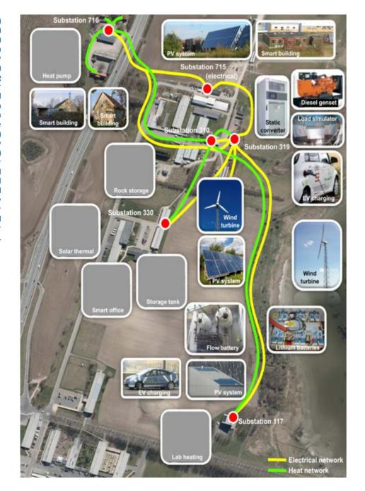
Figure 5. Lay-out and details of PowerLabDK/SYSLAB
